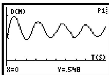
Figure 5. Graphics calculator graph of object suspended from a spring
